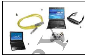
Fig. 1 The control unit: a) a personal computer (Asus G2S); b) a crosscable; c) a therapist's laptop (EEPC 100H - BK039X); d) A joypad (Xbox Controller); e) a head-mounted display (Vuzix iWear VR920)
